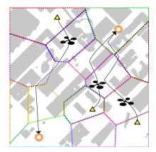
Fig. 1: The UAV traffic management problem. The airspace is divided into discrete sectors with a single UAV traffic management (UTM) agent controlling the cost of travel through each sector. UAVs traveling from start (triangle) to goal (circle) locations plan and execute paths to reduce their individual travel cost without explicitly coordinating with other UAVs in the airspace.
