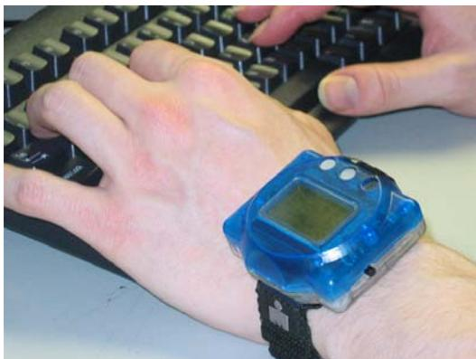
**Figure 1. eWatch sensor platform.**
