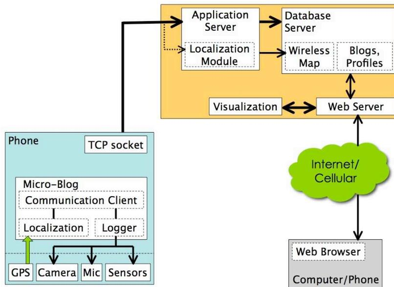
Figure 3: Block diagram of the Micro-Blog software architecture
