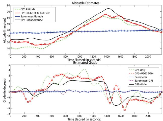
**Figure 6. (top) A plot of the estimated altitudes from GPS, Barometric, and GIS data sources. Note, that the Barometric pressure had an offset added to better illustrate how they all produce reasonable elevation profiles. (bottom) A plot of the estimated grades the person in Figure 6 walked on.**
