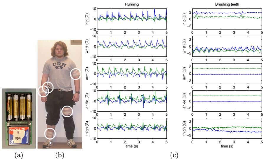
**Fig. 2.** (a) Hoarder data collection board, which stored data from a biaxial accelerometer. The biaxial accelerometers are attached to the opposite side of the board. (b) Hoarder boards were attached to 20 subjects on the 4 limb positions shown here (held on with medical gauze), plus the right hip. (c) Acceleration signals from five biaxial accelerometers for walking, running, and tooth brushing.
