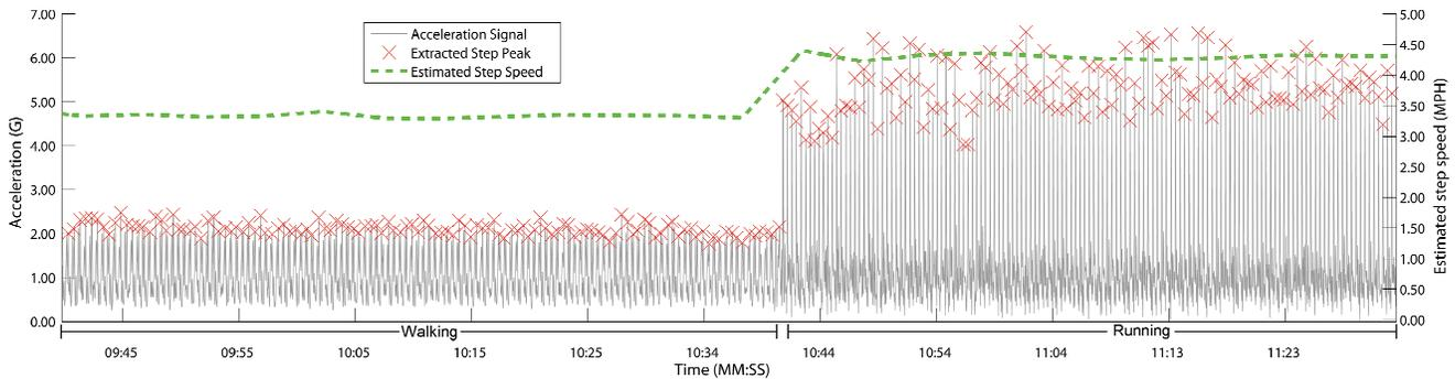
**Figure 4. Example accelerometer trace with the magnitude of the accelerometer shown in solid line at the bottom, extracted footfall peaks are marked with X's, and the estimated speed from the steps is shown as a dotted line. During the first half of the trace the subject was walking at around 3MPH and then began running at 4.5MPH near the 10:44 mark**
