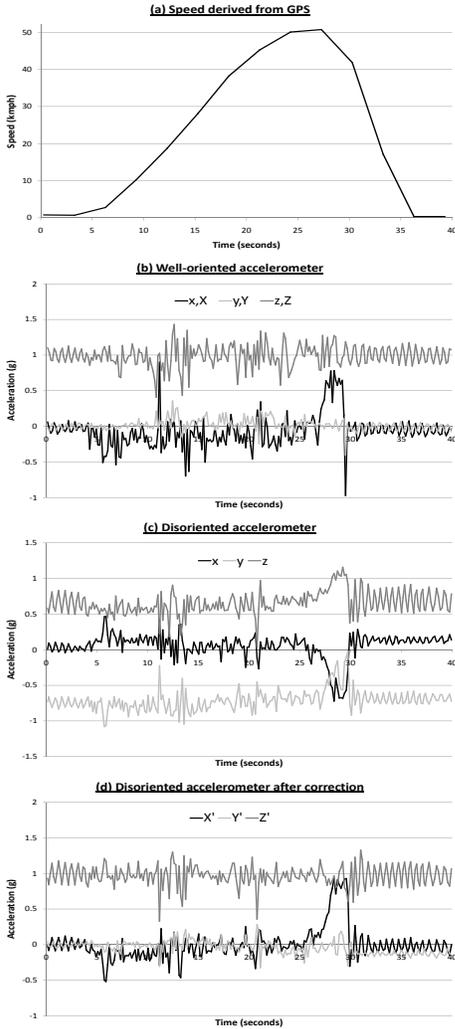
**Figure 4: Estimating the orientation of a disoriented accelerometer based on sharp deceleration starting at around 27 seconds:**  $\phi_{pre} = -88^\circ$ ,  $\theta_{tilt} = 49^\circ$ ,  $\psi_{post} = -135^\circ$
