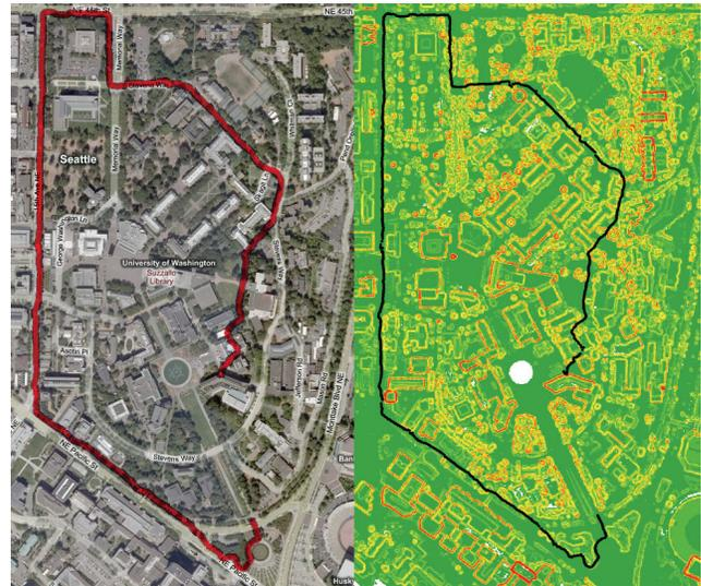
**Figure 5. (left) A GPS trace plotted on top of a satellite view. (right) A LIDAR slope contour plot of the same area, green areas have very little slope while red areas (like the edges of buildings) have large slopes.**
