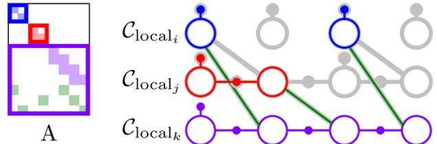
Fig. 1: Example factor graph estimation framework and corresponding measurement Jacobian,  $A$ . Each row of pose nodes (large circles) represents a single vehicle. The full (centralized) graph is highlighted in gray, while the reconstruction on board the third (purple) vehicle is fully colored.
